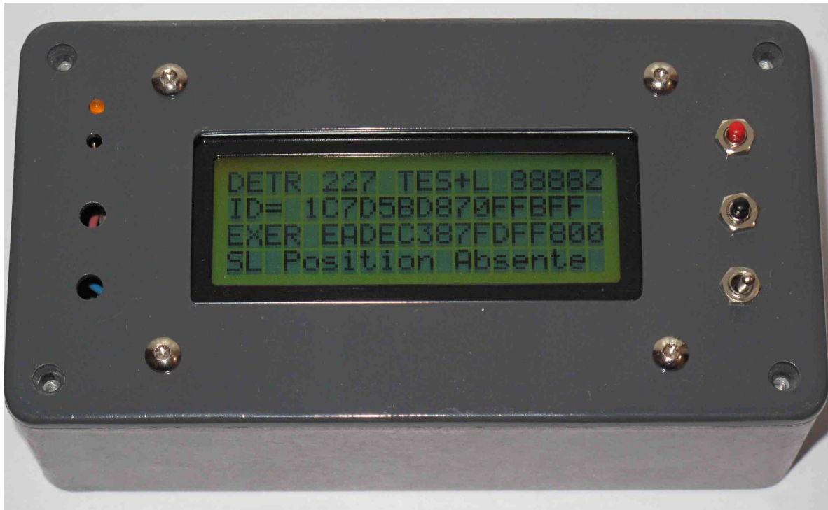
Photo E1: "4 lines decoder" in construction by F1AVR. Test with an Exercice Beacon
