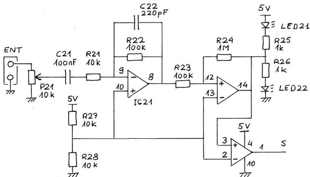
Figure 5: Diagram of input circuit
