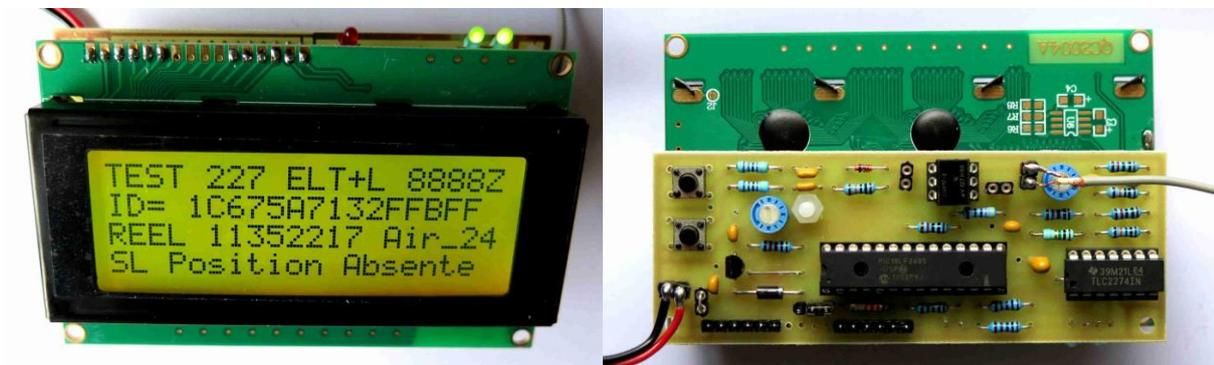
*Photo 1 and 2: The frame decoder with its new DECTRA PCB and display. Above the display, you can see the lighted green LED 2 for monitoring system operation.*
