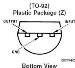
Figure 3: Pin assignment 78L05 5V 100mA regulator
