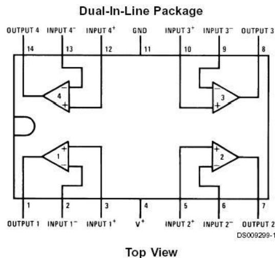
Figure 2: Pin assignment TLC2274 (classic pin for a quad op amp.)
