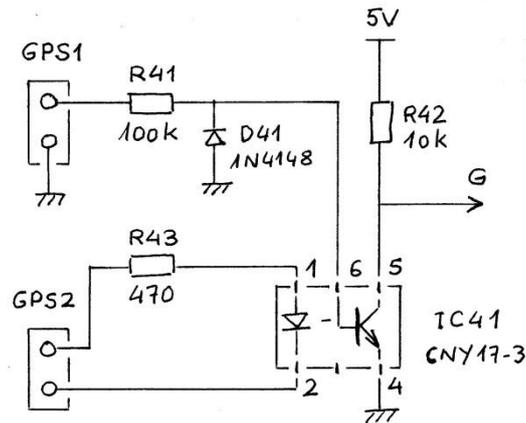
Figure 7: Schematic of the GPS input
