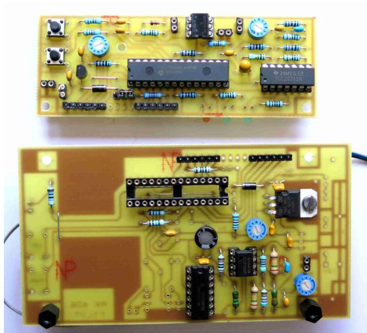
*Photo 3: Comparison of the size of the DECTRA PCB (top) to that of the original PCB (bottom, partially wired)*
