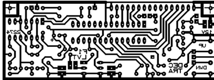
Figure 1: PCB component side seen at scale 1:1
