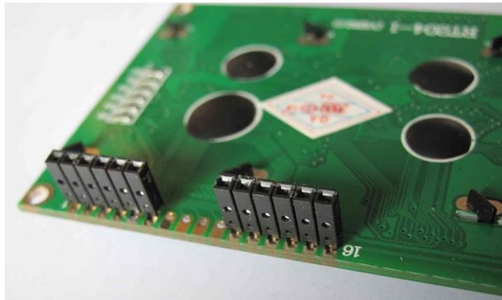
*Photo 7: 2 female 6 pin connectors soldered under the display*
