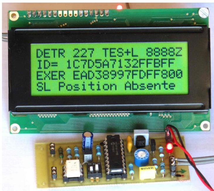
*Photo 10: The decoding of an "Exercise" frame from a frame generator.*
